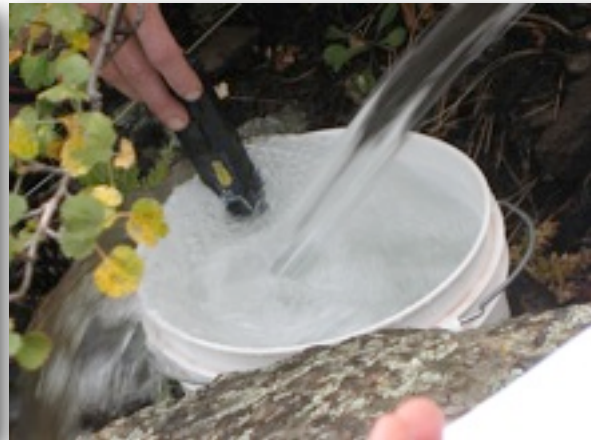
Figure 3. PVC extension attached to Big Leroux Spring drain pipe for the purpose measuring spring flow with a bucket.
