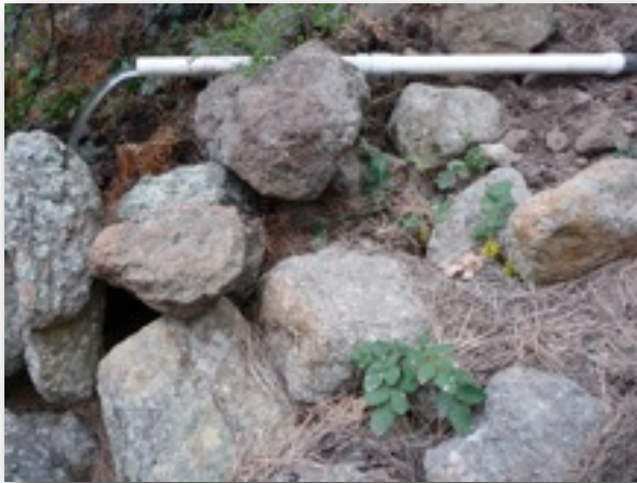
Figure 3. PVC extension attached to Big Leroux Spring drain pipe for the purpose measuring spring flow with a bucket.
