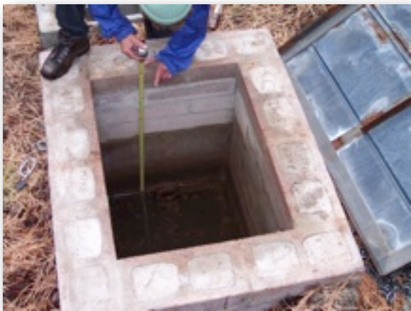
Figure 4. Measuring from top of Big Leroux Spring box to water surface.
